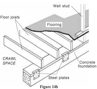
**Figure 14**—**Anchor bolts or steel plates.** A home's crawl space may be formed by a cripple wall *(see next page for description)* between the foundation and the floor joists or the floor joists may rest directly on the sill plate. In either case, you should be able to see the heads of anchor bolts or steel plates installed at appropriate intervals. These fixtures fasten the sill plate to the foundation.
