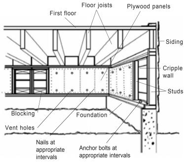
Figure 17—Plywood or diagonal sheathing strengthens weak cripple walls. If your home has a cripple wall between the foundation and the first floor, and the wall is not braced with plywood or diagonal sheathing, the house may fall or shift off its foundation during an earthquake.
