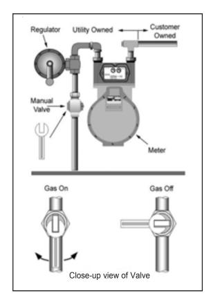
Figure 36—Manual Shutoff Valve Location
