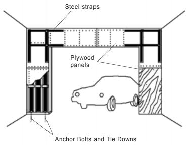
**Figure 32—Bracing garage walls.** If your house has a room over the garage, the garage walls may not be strong enough to hold up during an earthquake unless they are braced with plywood panels and steel straps.
