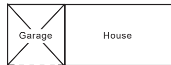
Figure 30 - If the wall of the main house is in line with the wall containing the door of a garage with a room over it, the adjoining wall may help brace the garage.
